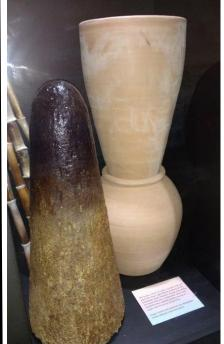
Sugar cone clay mold; the tip has a small hole so debris and molasses can flow through into the kettle.
